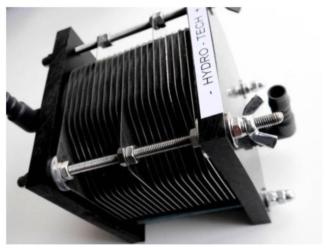
Solution connections . All connections need to be secured with cable ties etc. Hose need to be made out of acid resistant materials only ( silicone for example ) otherwise may melt due to be subject to acid like solution . Please make sure that if solution will make contact with skin You will immediately wash Your hand with soap using warm water .
